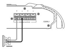
Figure 3. CS subwoofer amplifier with one woofer connection.
